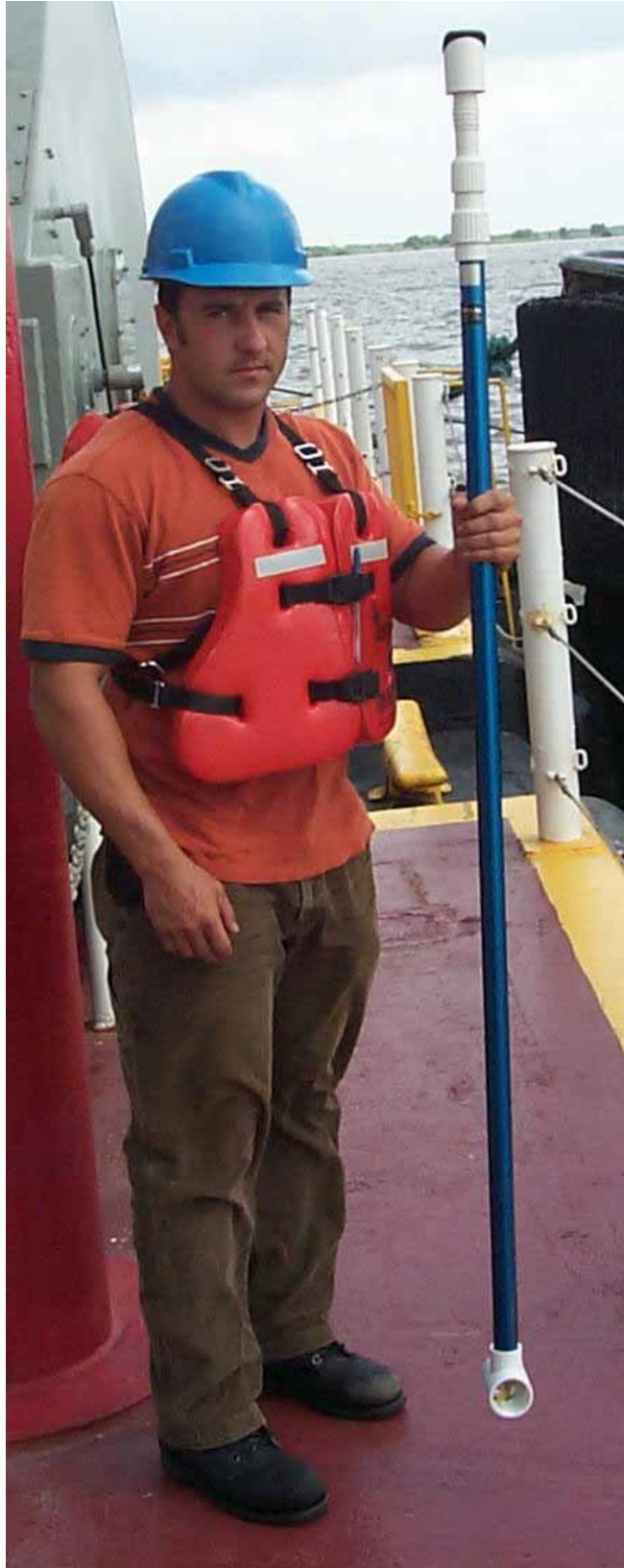
Photo 27. FP201 Global Flow Probe (wand not extended)
