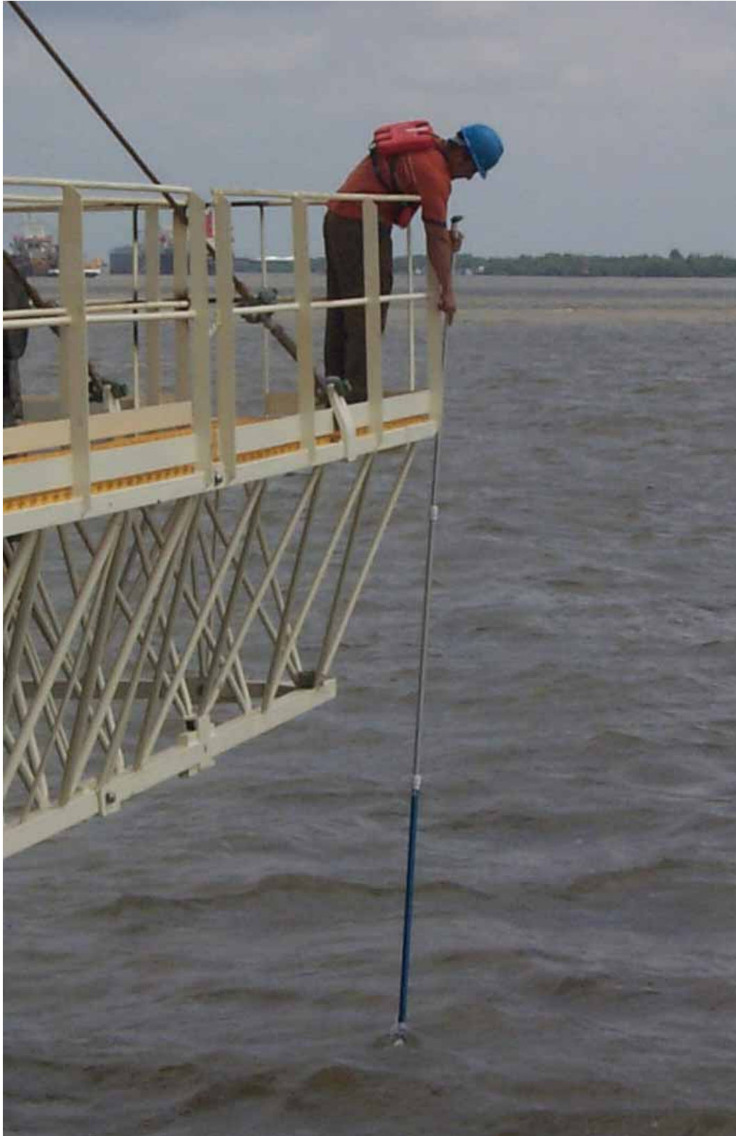
Photo 28. Current meter being deployed off Beachbuilder's bow gantry
