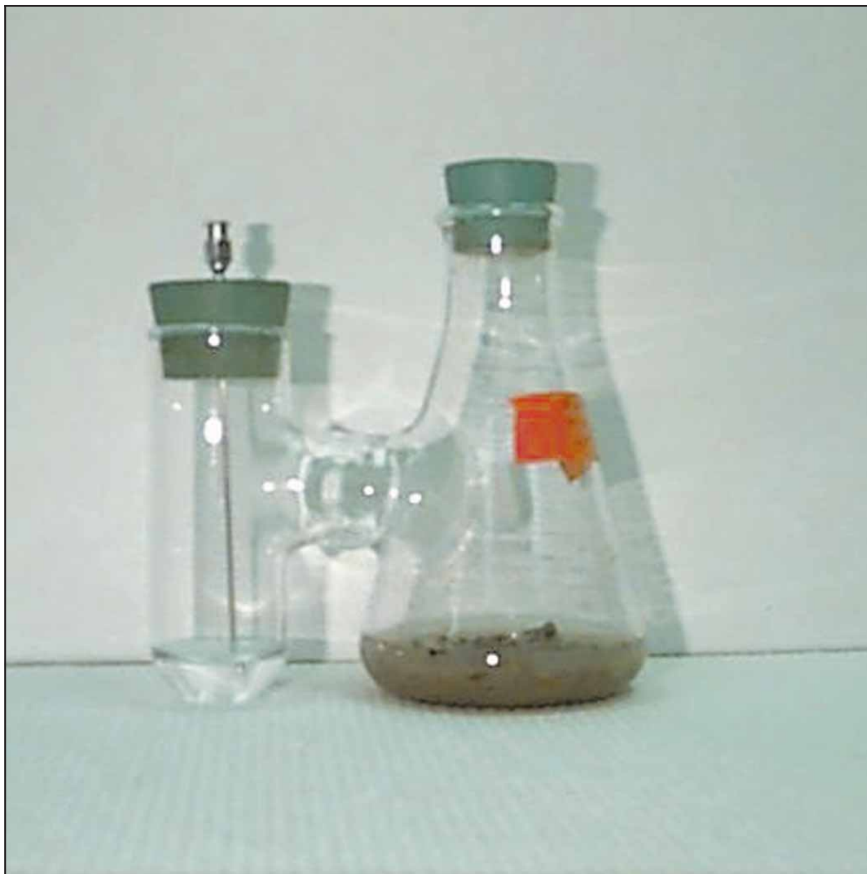
Figure 5. Biotreatability micocosm consisting of a 250-ml biometer flask containing 50 ml of a sediment slurry (30 percent wet/vol) (The flask is placed on an orbital shaker to continually mix and suspend solids. The same vessel can be used for radiorespirometry studies. In these studies, approximately 800,000 cpm of the radio-labeled contaminant is mixed into the sediment slurry, and 2 ml of 1 M KOH is placed in the side arm well to trap 14 CO 2 )
