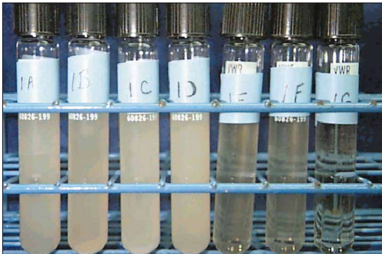
Figure 3. A seven tube most probable number dilution series showing turbidity and gas production as a result of microbial growth
